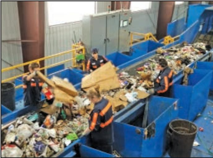
**Recyclable cardboard is manually removed from waste stream**
