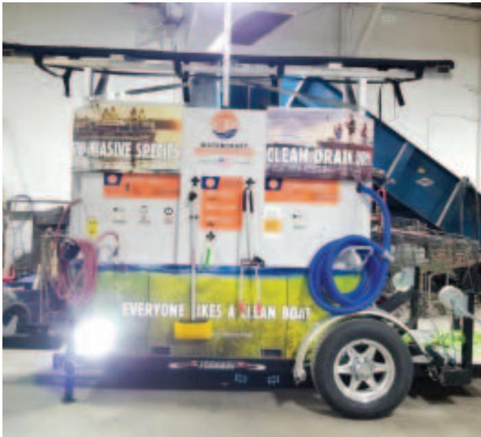
Solar-powered boat cleaning unit
